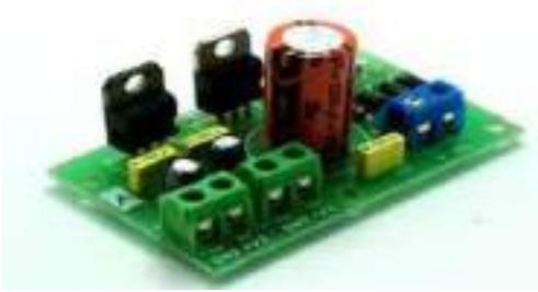
**Fig.5. Power Supply Board**
