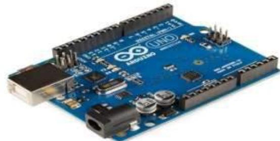
**Fig.4. Arduino Board**
